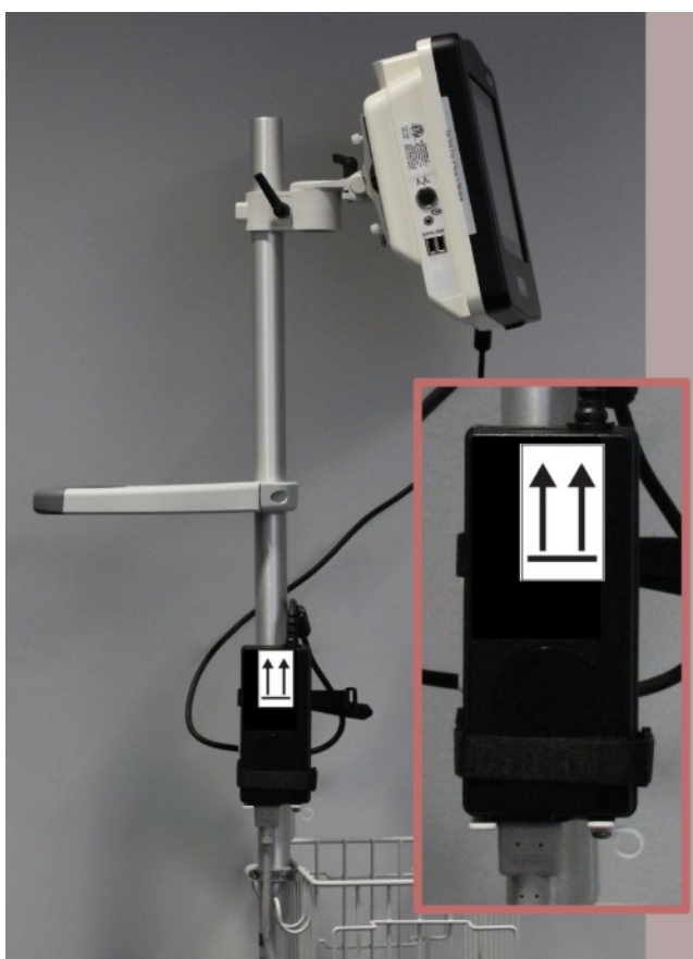
Fig. 1-2: Power supply shown mounted correctly, with arrows pointing upward
