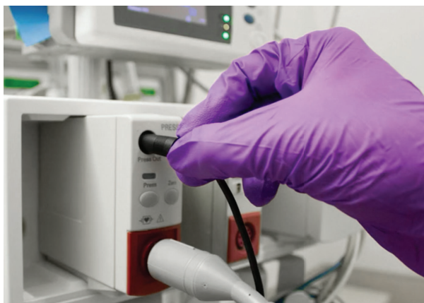
The Argos connects to the analog output of the IBP signal from a compatible bedside monitor
