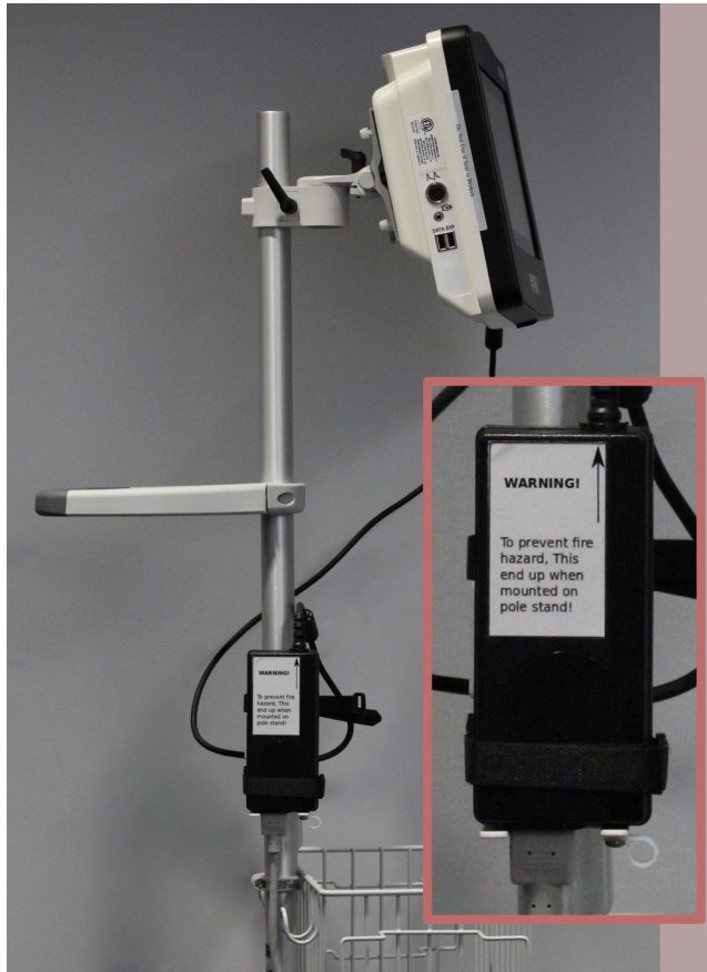
Fig. 6-2: Power supply shown mounted correctly, with arrow pointing upward
